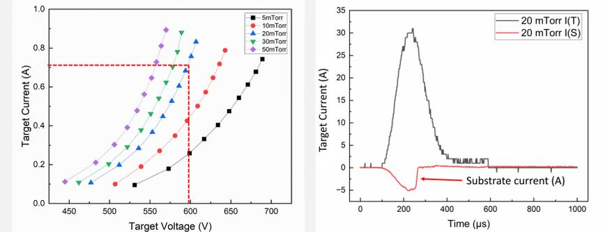
Higher working pressure results in higher target current for a given voltage
