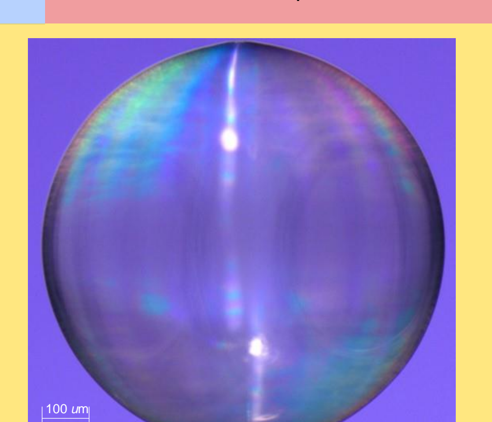
A concept target with an 850- \mu\text{m} OD capsule and an 8- \mu\text{m} wall, was printed for future use on OMEGA; a 50- \mu\text{m} drain hole was added to the print to allow for resin drainage
