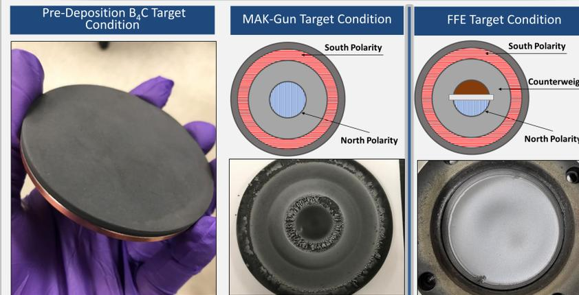
Redeposition of "dust" from plasma onto target virtually eliminated with FFE.
