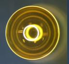
3.15mmx8.8µm SiCH (6at% Si) capsule after 1 atm buckle test
