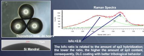
The  $I_D/I_G$  ratio is related to the amount of  $sp^3$  hybridization; the lower the ratio, the higher the amount of  $sp^3$  content, consequently, DLC coating with better tribological behavior
