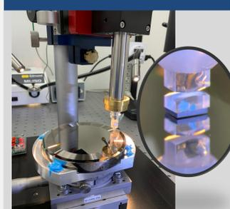
EOS brick being glued down for Diamond turning process
