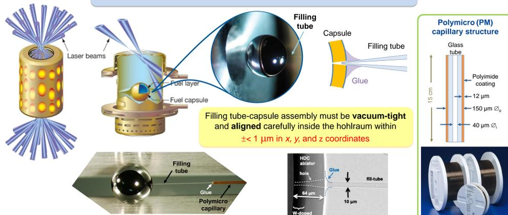
Filling tube-capsule assembly must be **vacuum-tight** and **aligned** carefully inside the hohlraum within  $\pm 1 \mu\text{m}$  in  $x, y,$  and  $z$  coordinates
