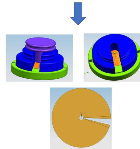
A combination of forming the shield in place and securing the ends of the shield blank together with glue was used to produce the conical shield components.
