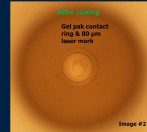
Image #2: A 80 μm fiducial with a gel pak contact ring is observed on the top surface of an 860 x 25 μm GDP capsule after coating.
