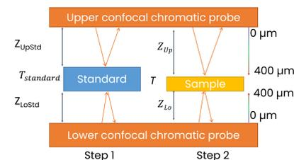
Step 1: The distance separating two probes is estimated by using a thickness standard ( $T_{standard}$ ,  $Z_{UpStd}$  and  $Z_{LoStd}$ ).Step 2: The sample is placed instead of standard ( $Z_{Up}$  and  $Z_{Lo}$ ).
