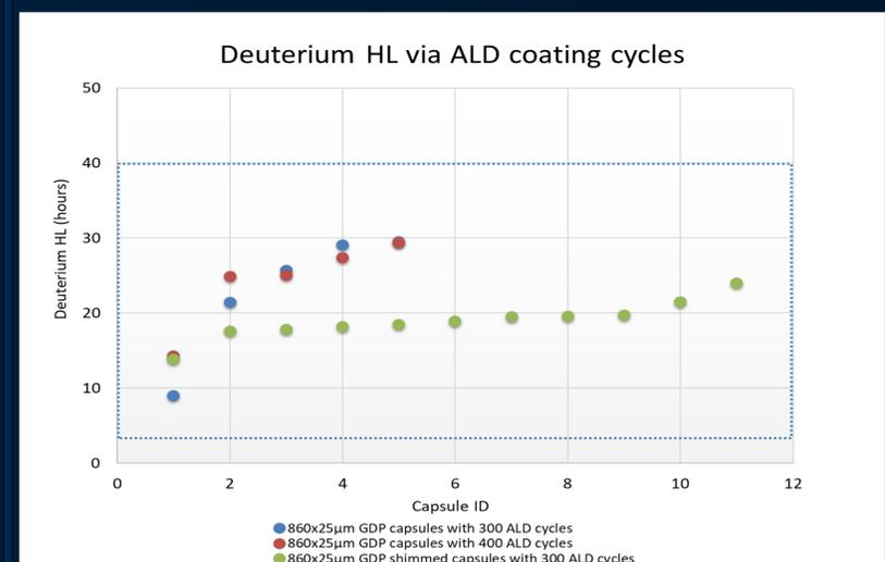
**Aluminum (Al) coating:** typical GDP capsules have a  $0.1 \pm 0.03 \mu\text{m}$  aluminum (Al) coating to retain gas, providing a deuterium HL of 2.7 to 40 hours. However, the opaque Al coating obstructs the 80 μm fiducial, making alignment and mounting difficult in the OMEGA system. To address this, we explored using a transparent SiO<sub>2</sub> layer by ALD as a gas-retentive barrier for the shimmed capsules.
