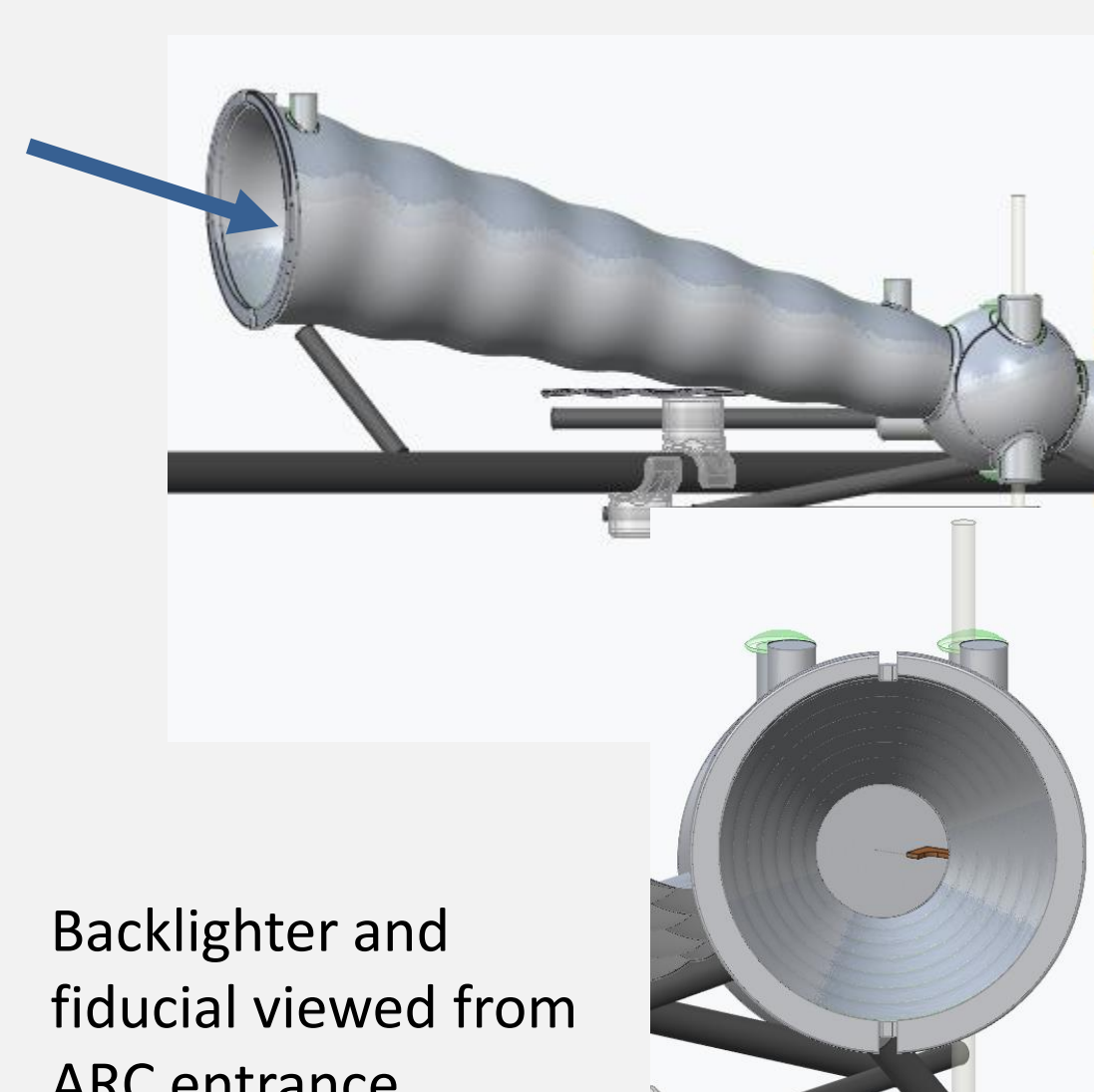
Wire is not measurable after shield caps are installed
