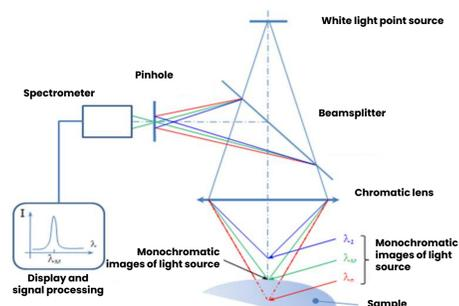
Thus, sample surface position or transparent object thickness is accurately determined in the measuring field.
