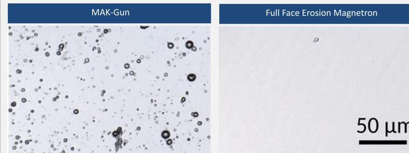
Confocal micrographs show the contrast in nodular defect density between MAK and FFE sources.
