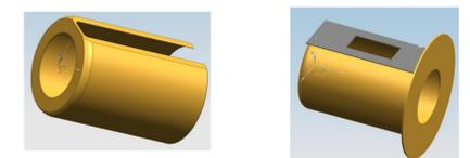
The hohlraum body will be produced using standard manufacturing processes with an additional machining stage to produce the slot along the length of the component. The flat foil with a square hole and the end cap will be laser machined and then assembled to the hohlraum body. This is being trialled as part of R&D ahead of final target production to prove out the manufacturing process (Machining and assembly).
