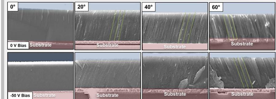
Redeposition of dust from plasma onto target significantly reduced with FFE.
