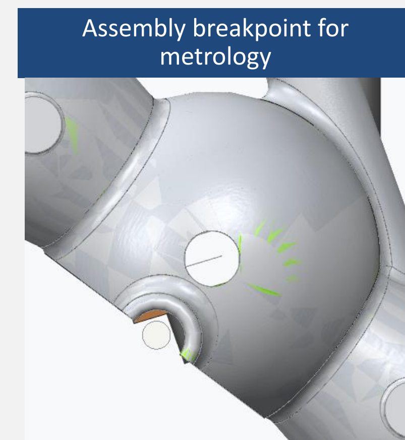
Wire is measured through metrology viewing window
