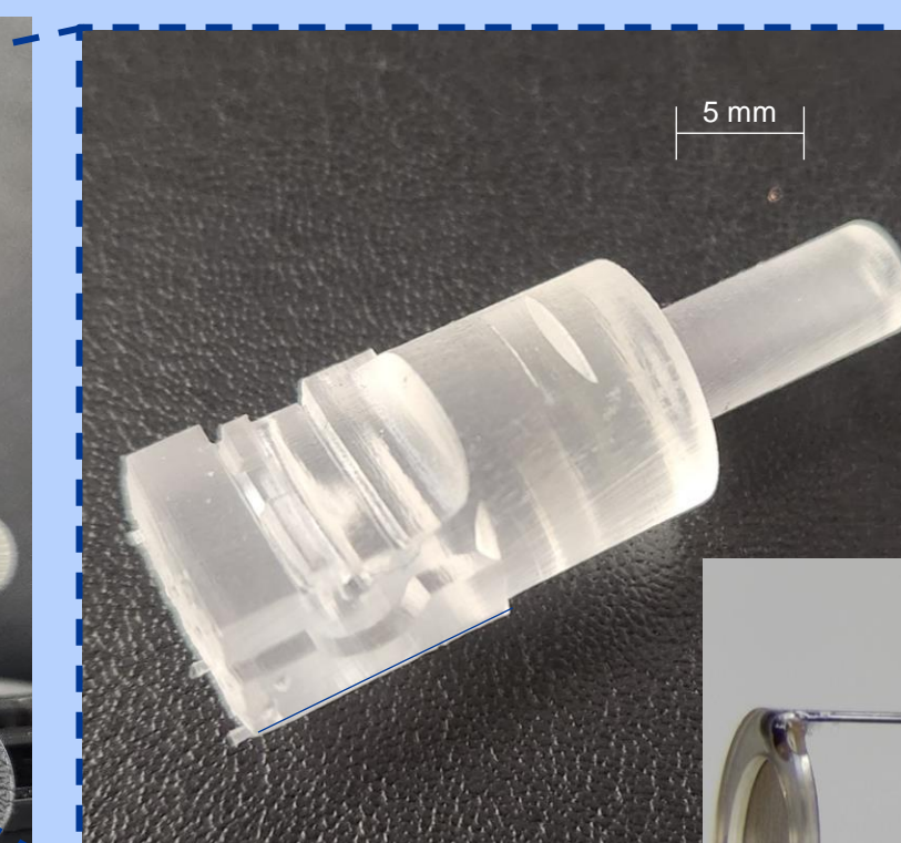
A fixture holds a strainer to allow printed parts to be removed from their substrates and soaked in isopropyl alcohol in a controlled manner
