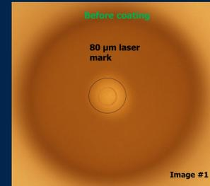
Image #1: A 80 μm fiducial with a step height of approximately 0.4 μm is visible on the top surface of an 860 x 25 μm GDP capsule before coating.
