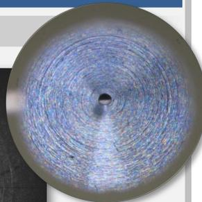
TFAB PICMET Image of pinhole aperture through mirror
