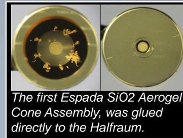
The first Espada SiO2 Aerogel Cone Assembly, was glued directly to the Halfraum.
