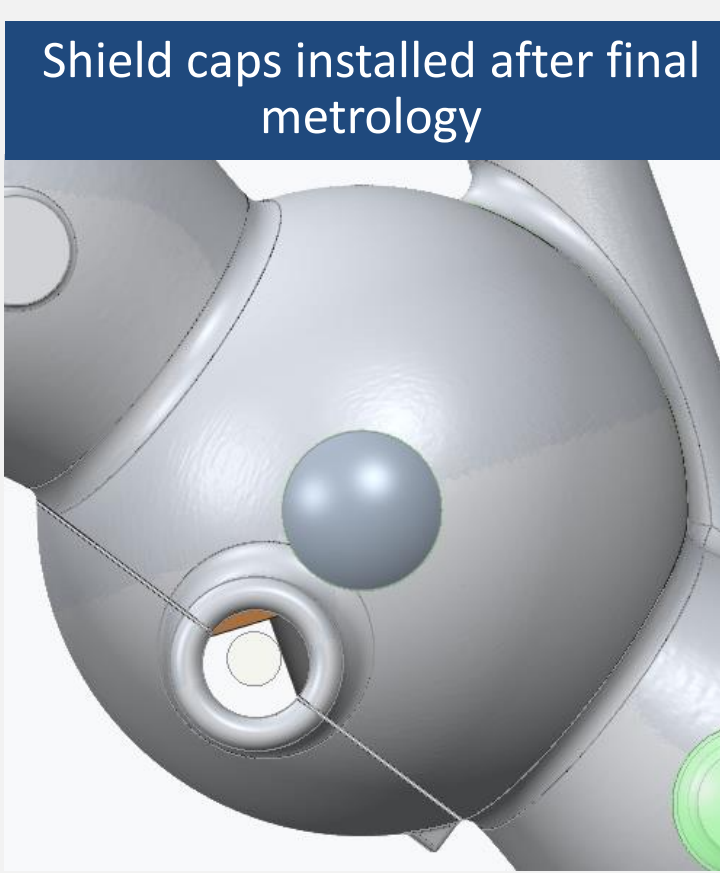
Wire is not measurable after shield caps are installed
