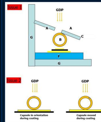
Keeping the 80 μm fiducial at the top/bottom center during coating is crucial. However, two major issues reduced the coating yield of shimmed capsules.
