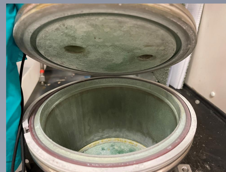
Interior of original pressure leaching vessel
