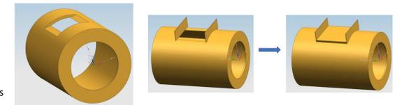
An alternative design was proposed; however, it was not favoured due to the tight tolerances/fits which would be required to assemble the layer pack in the correct position. This design included the use of foils positioned at either end of the layer pack:
