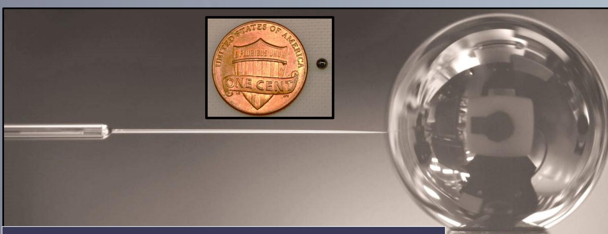
Fill Tube and capsule close-up profile
