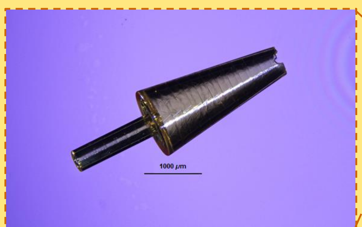
The fixture is 4 mm total in length with a 100- \mu\text{m} -thick wall, and a 1.6-mm-long, 100- \mu\text{m} -diameter vacuum channel fits inside the bore of a vacuum chuck
