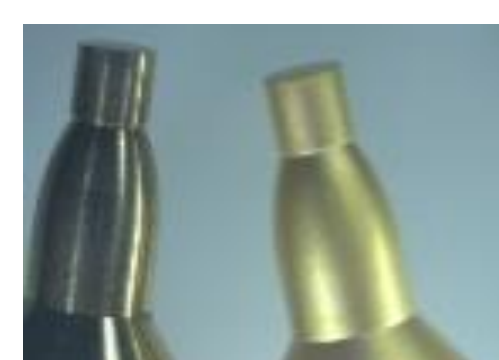
Mandrel before and after thin gold plating
