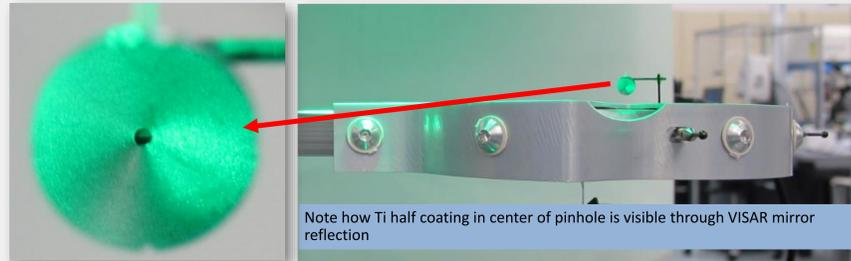
VISAR mirrors are used when we want to make VISAR measurements **without** the line of sight facing VISAR (90°-315°)
