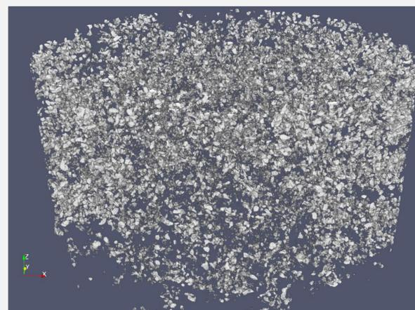
Chunk Mix consisting of 60 μm particles dispersed in a 50 mg/cc CH matrix at 20% by volume prior to machining and assembly
