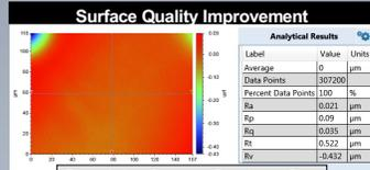
Example Interferometry Roughness Data
