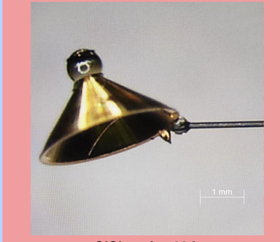
CISImprint-23A Part number Q-FA-C-498 are gold-coated cones with a 500 \mu\text{m} opening to seat a drilled capsule
