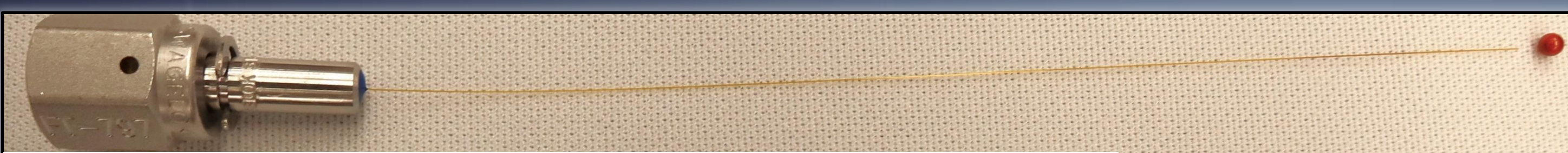
CFTA main assembly components: capsule, fill tube (FT) and polyimide sleeve attached to a VCR female fitting
