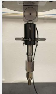
(Left) 5 N Load cell with custom fixturing to directly mount CFTA with VCR fitting
