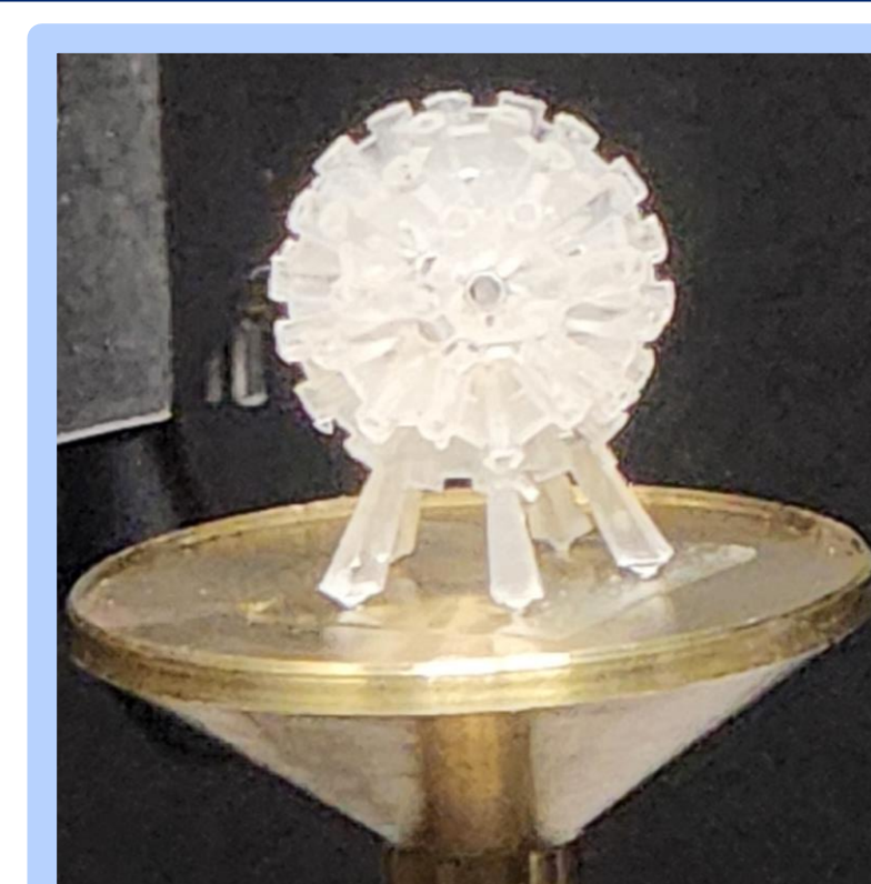
Printed on the Formlabs Form 3 printer; this 12-mm-sized replica of the OMEGA chamber was used to test electroless copper plating; the part was then imaged on the Bruker Skyscan221 XRM
