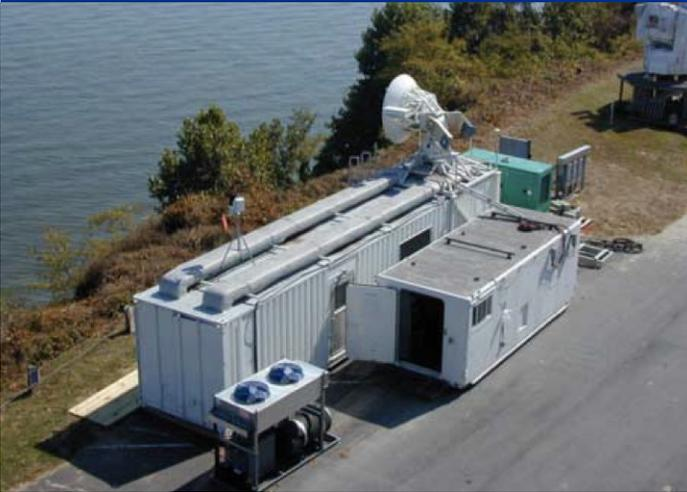
*This proof-of-concept long-range radar transmitter used for imaging aircraft produced a 10 kW amplified signal with nearly 1 GHz bandwidth at 94 GHz. (Naval Research Laboratory)*
