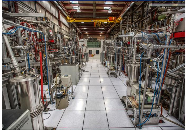
*This first-of-its-kind high-power microwave system delivers over 4 MW at 110 GHz in a 10 s pulse length. New waveguide components from GA have been designed for steady-state MW-level conditions from 110 to 170 GHz. (Department of Energy)*
