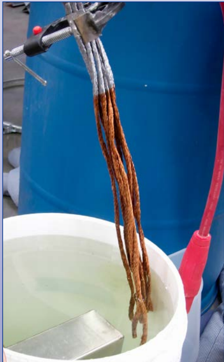
Conductor strands after chrome stripping
