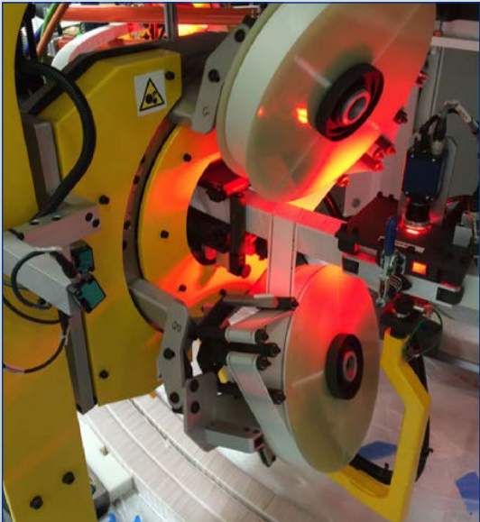
Automated heads wrapping fiberglass tape around the conductor
