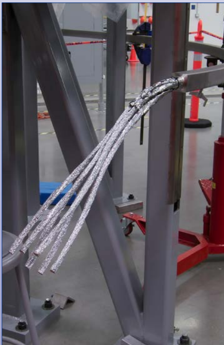
Conductor strands prior to chrome stripping
