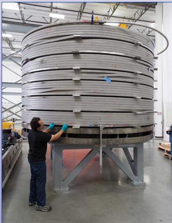
Module with six completed splice joints
