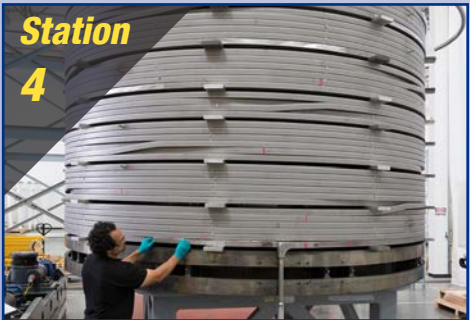
Stack & Join/Helium Penetrations
