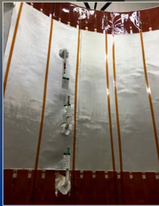
Helium inlet pipe with ground insulation
