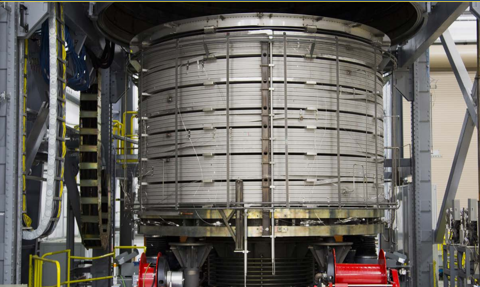
Placing module in furnace for heat treatment at 650°C (1200°F)
