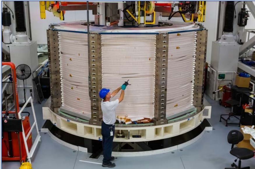
Turn insulation of module nearing completion
