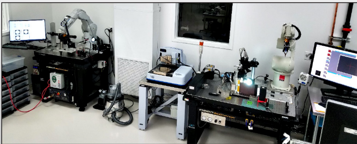
Automated shell characterization and sorting line uses machine learning
