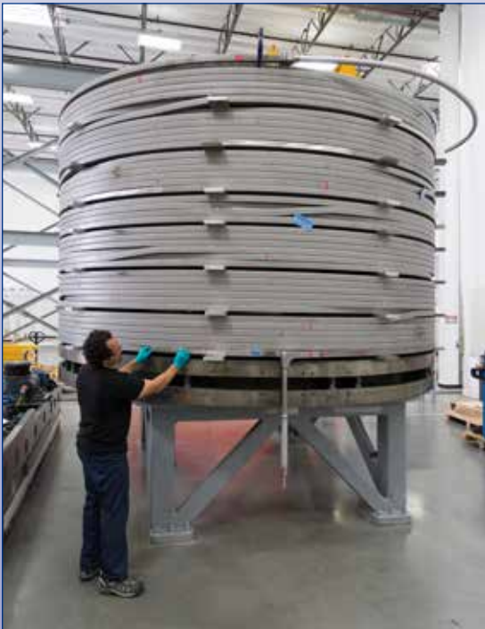
Module with six completed splice joints
