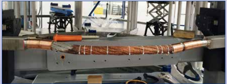
Splicing the conductor cable together similar to splicing a rope
