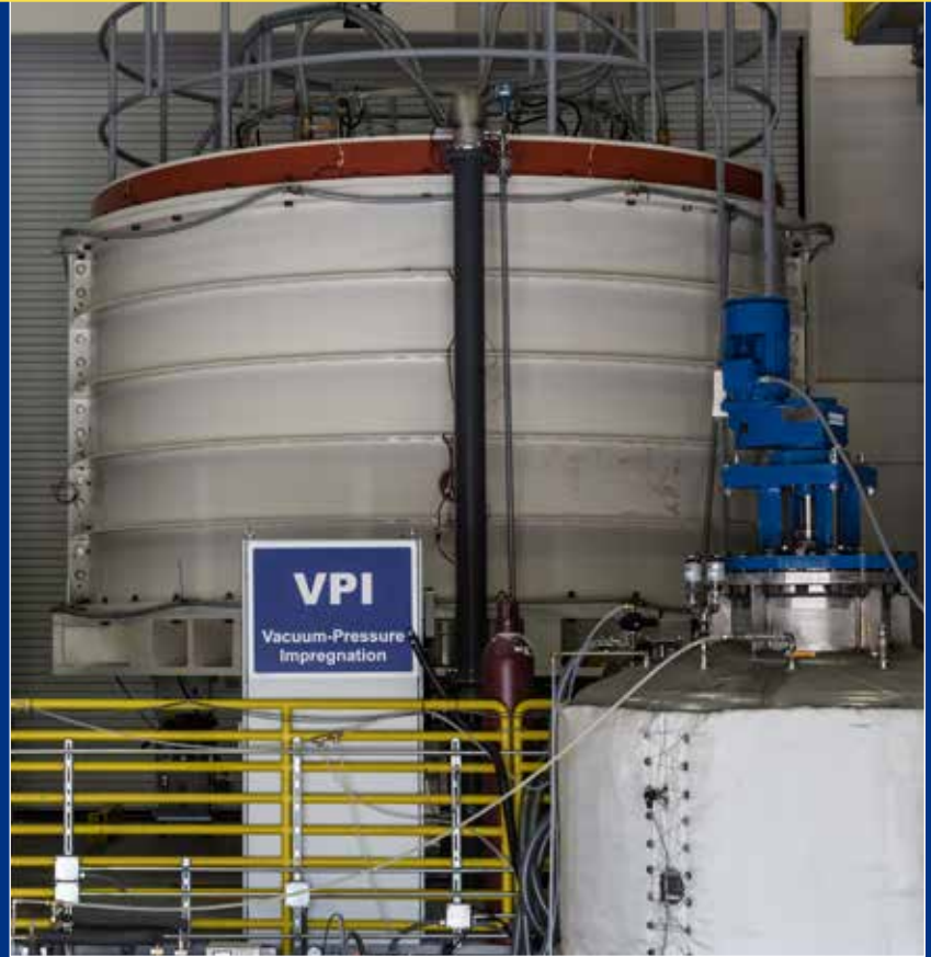
Module mold alongside resin tanks and mixing pump system for injecting 3,500 liters of resin to encapsulate the module
