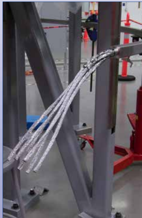
Conductor strands prior to chrome stripping
