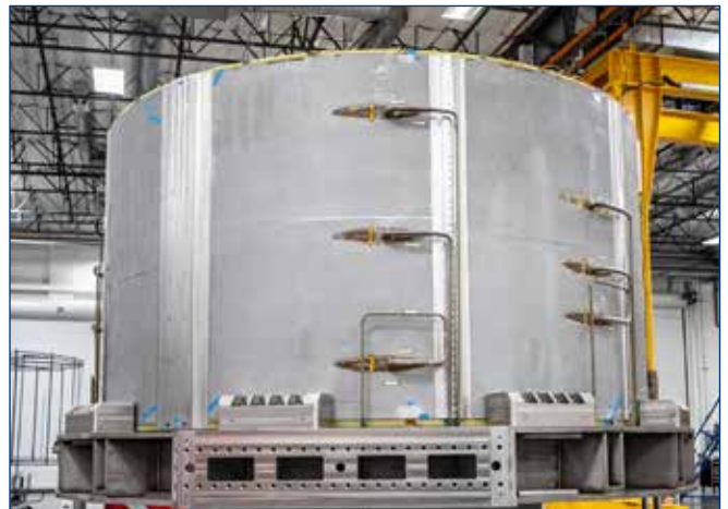
Module after piping installed
