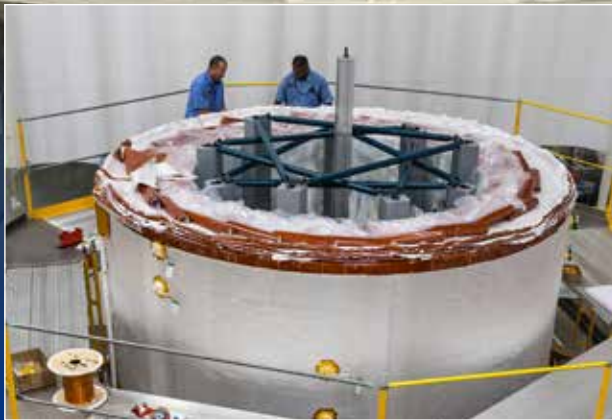
Module during ground insulation application
