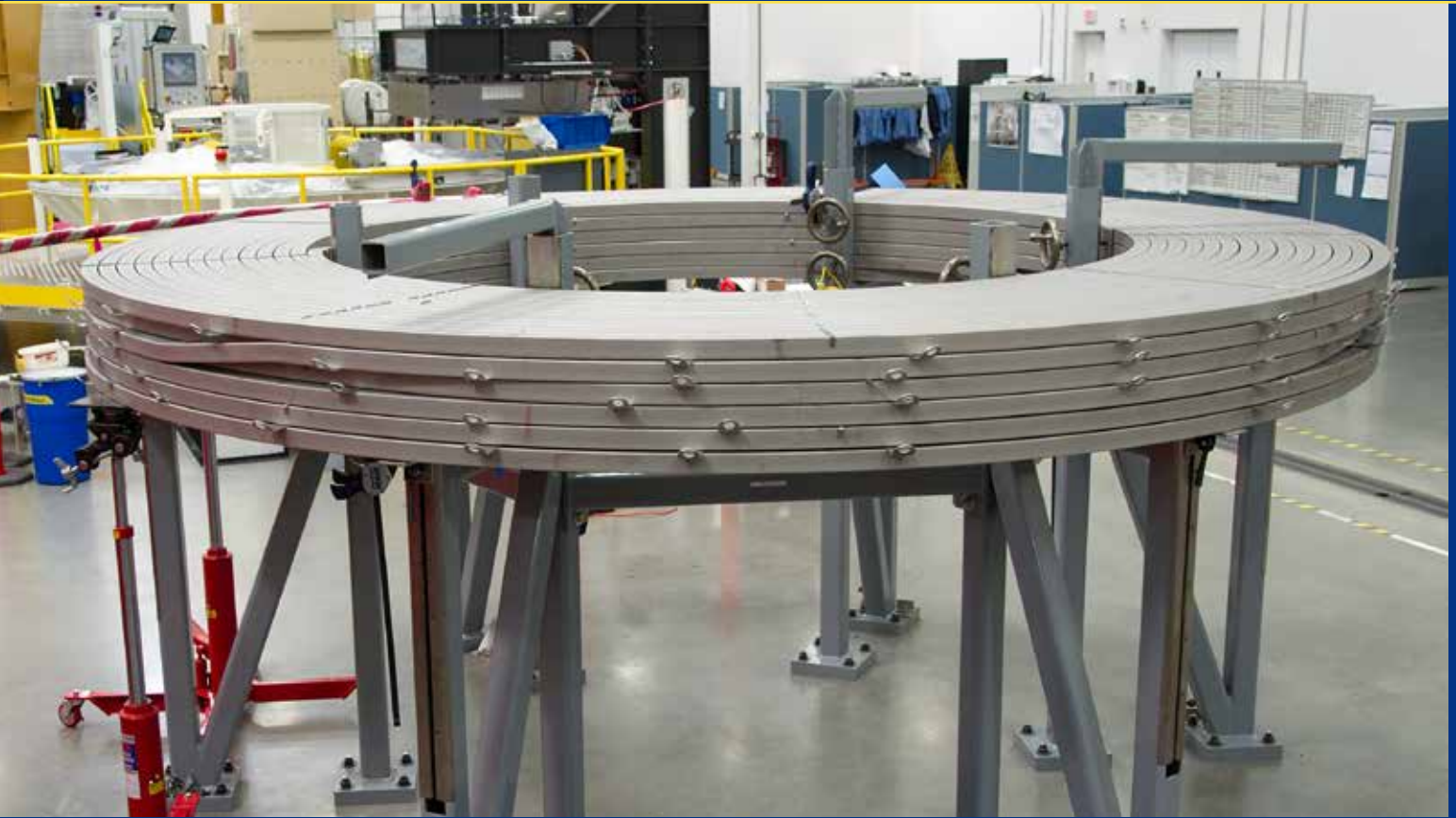
Wound six-layer submodules ready for terminal preparation
