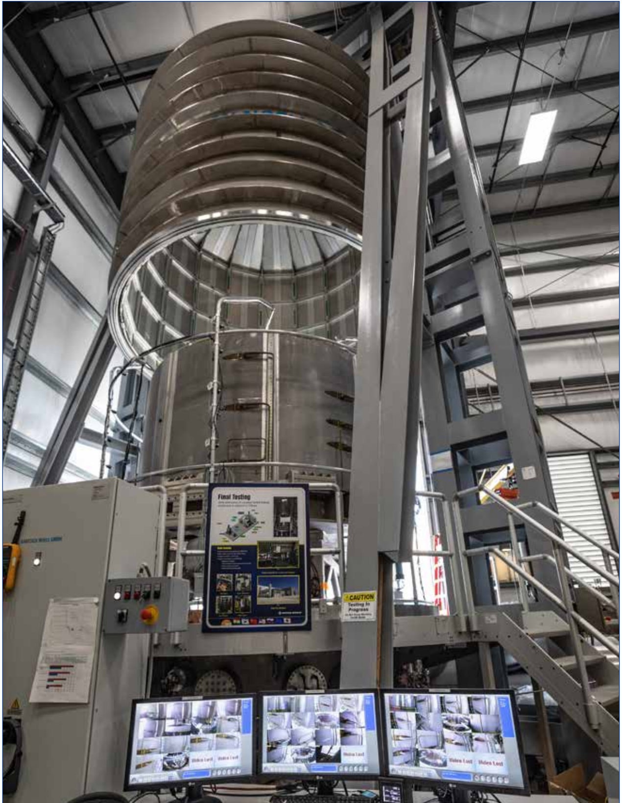
Module in final test chamber with camera system installed ready to begin high voltage testing
