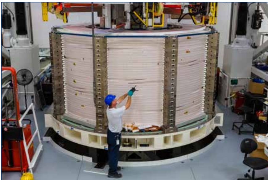
Turn insulation of module nearing completion
