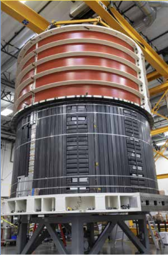
VPI mold being placed over the module in preparation for resin injection
