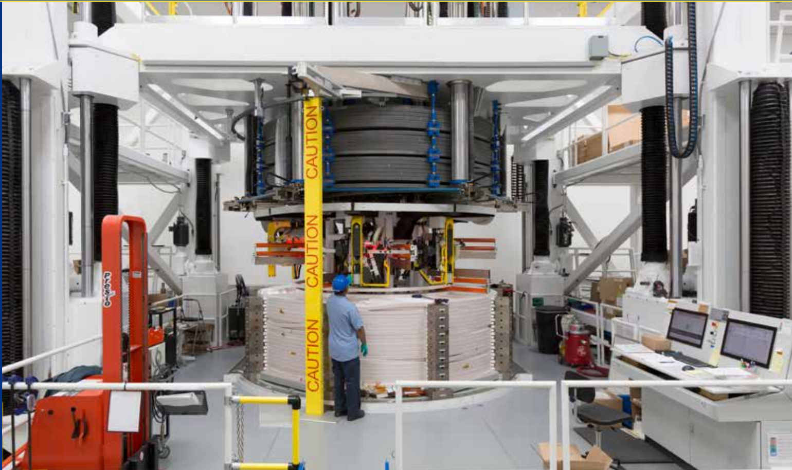
Turn insulation station structure lifts and raises 110-tonne module and releases individual turns for insulation wrapping
