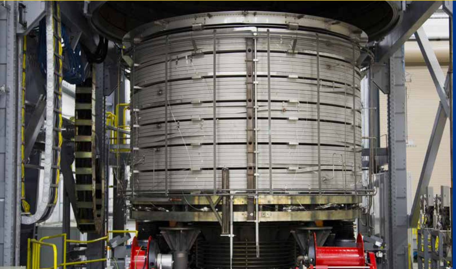
Placing module in furnace for heat treatment at 650°C (1200°F)
