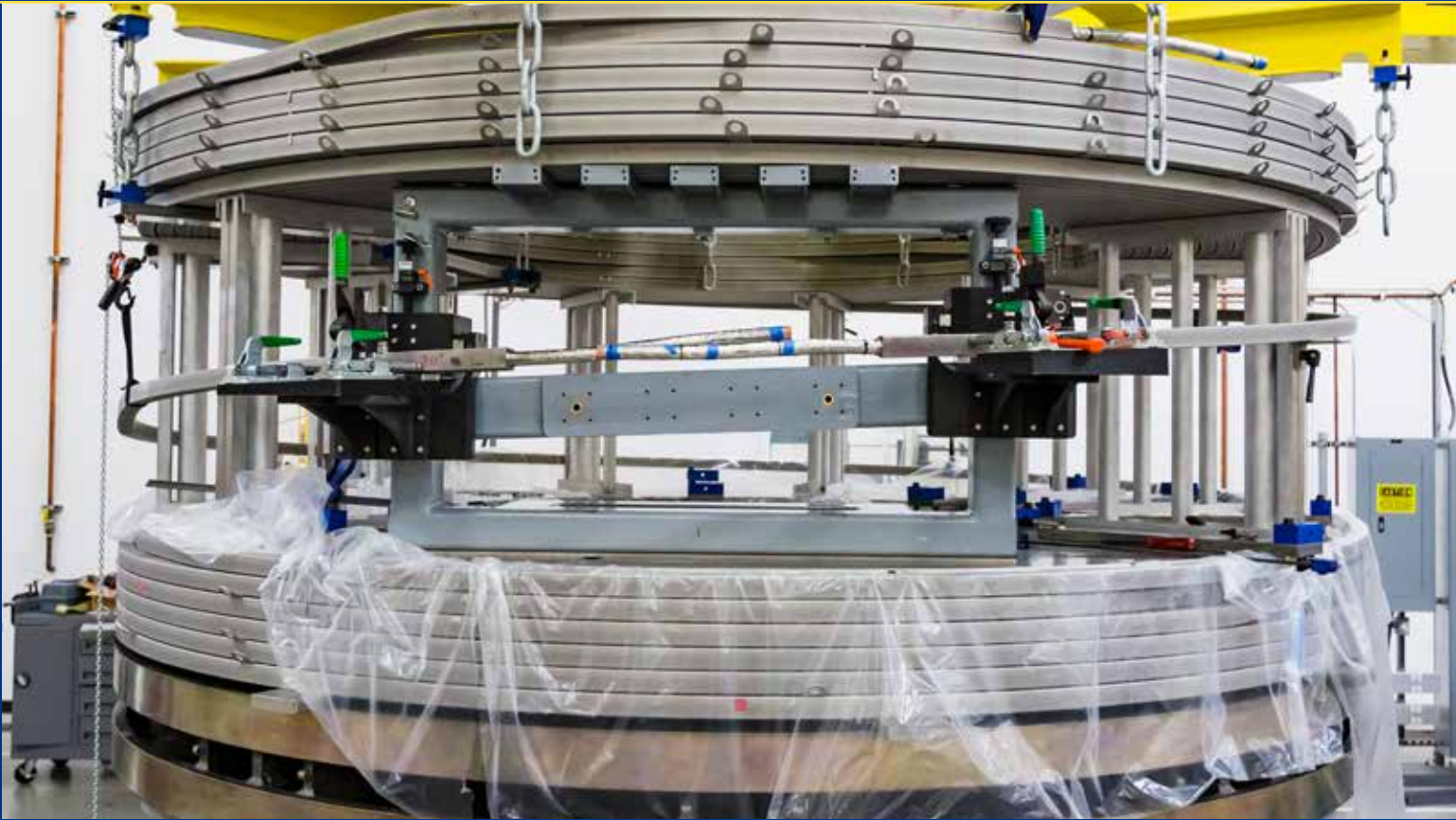
Two hex submodules prepared prior to joining
