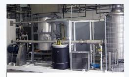
3 GPM Super-Critical Water Oxidation (SCWO) skid
