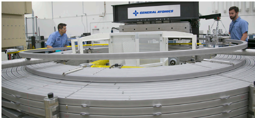
Superconductor is wound to high tolerance
