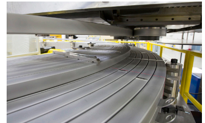
Superconductor is wound to high tolerance
