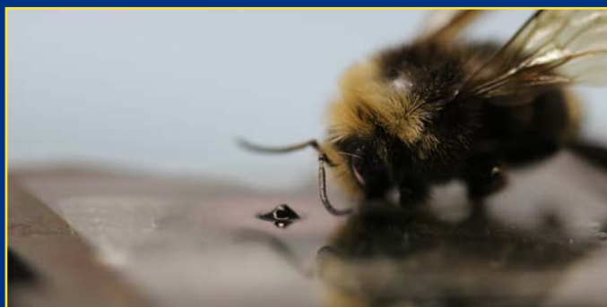
Sub-millimeter mound of copper aerogel applied with a GA-developed nanoparticle deposition system
