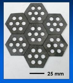
Plates with integral hole pattern
