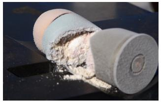
40mm HEPD grenade post cryofracture processing
